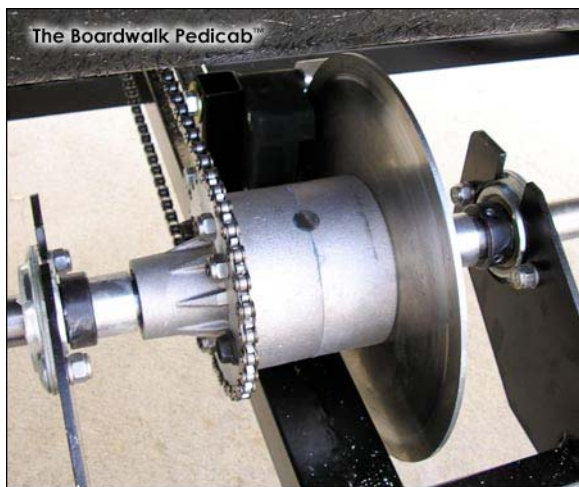
Braking is provided by a revolutionary hydraulic 8-3/4" rear disk brake and supported by a front V brake.
