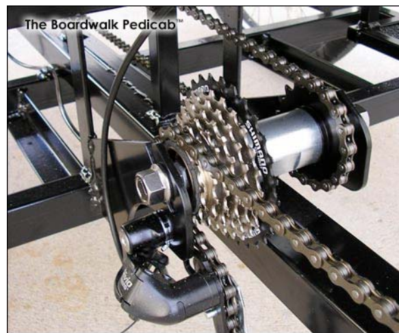
All Boardwalk Pedicabs™ features a Shimano 21-speed drivetrain with a rear axle differential and indexed, grip-shifting.
