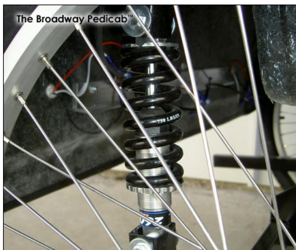
Adjustable coil spring shock provides excellent road dampening and a smooth ride for your passengers.
