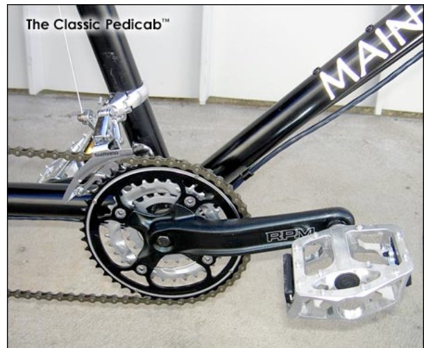
All Classic Pedicabs™ feature a Shimano 21-speed drivetrain with a rear axle differential.
