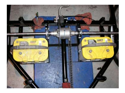
Each battery has four holes along the base, 2 in the front and two in the back
