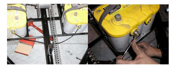
Step 2: Attaching black/negative cables to negative terminal on left side battery
